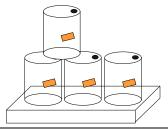
**CASE 3:** The capacity of the containing basin should be 25% of the total volume of the drums.
