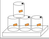
**CASE 3:** The capacity of the containing basin should be 25% of the total volume of the drums.
