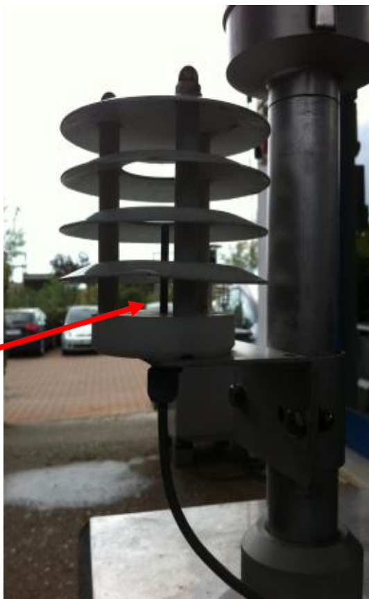
Figure 13: Detail of the atmospheric pressure and temperature sensor
