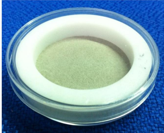
Figure 6: Petri Dish containing a filter cassette and an exposed filter
