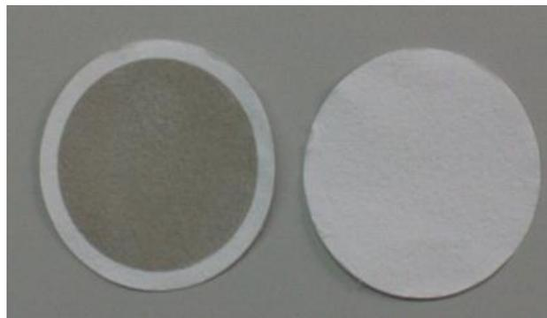
Figure 7: Exposed Filter (left) and Unexposed Filter (right)
