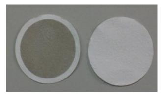
Figure 7: Exposed Filter (left) and Unexposed Filter (right)
