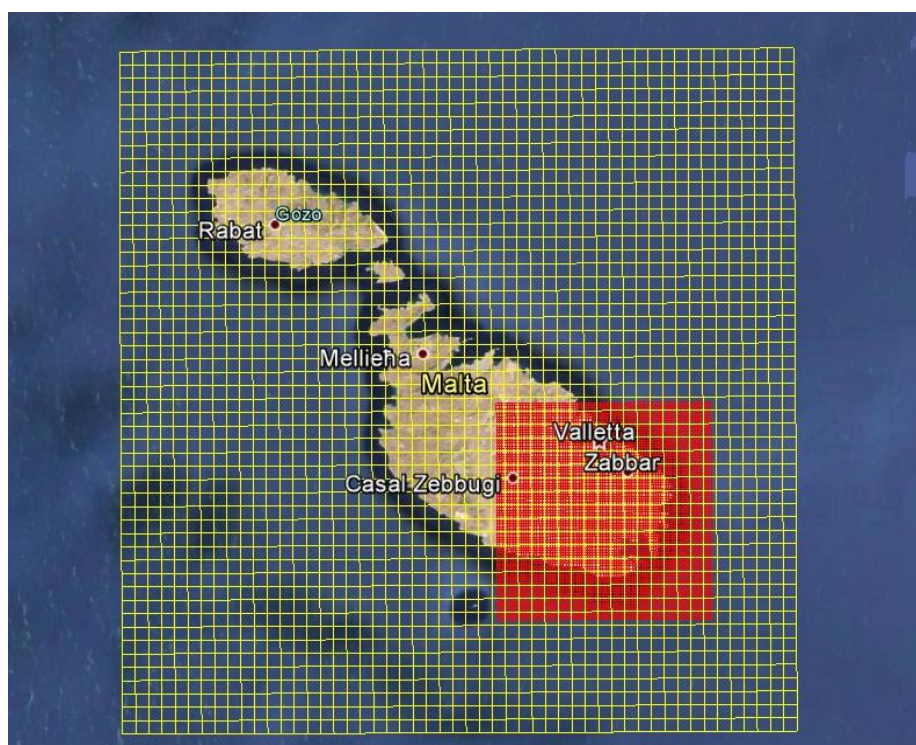
Figure 4. Computational grid used to describe the background concentrations through the CTM model, covering the entire Maltese Islands with horizontal resolution of 1 km. The inner red square represents the localization of the LPDM local domain.
